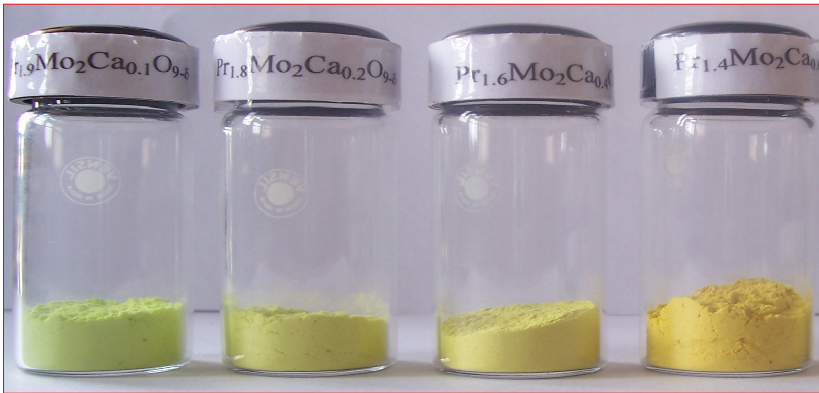
Photographs of samples of environmentally benign yellow pigments produced by the group.
